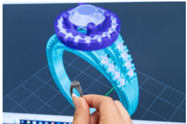
Students use CAD software and 3D printers as a rapid prototyping system to design & manufacture jewelry - ©GIA
