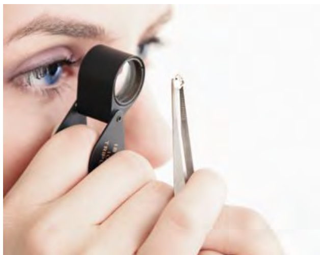
Diamond Grading Lab students assess a diamond's clarity using a 10X jeweler's loupe - ©GIA
