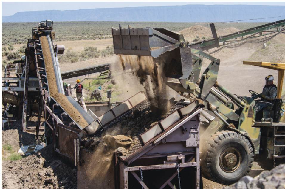
Figure 13. Dust Devil uses heavy-duty excavators to mine the basalt ore, which is processed by a grizzly (a grille with evenly spaced bars to exclude larger rock). The basalt ore then passes through a sequence of conveyors to a shaker, a wet trommel, a hopper, and a belt for handpicking. Some of the ore goes to an optical sorting machine, depending on the mine's production needs. Photo by Robert Weldon.
