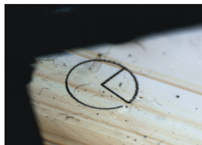
Figure 8. The 0.9 mm diameter laser manufacturing remnant on this diamond showed an interesting pattern.
