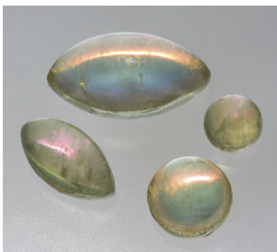
Figure 1. These assembled cabochons (1.74–10.57 ct) with multi-color iridescence are a skillful imitation of rainbow moonstone. They are composed of a natural rock crystal quartz base with an iridescent coating cemented to a gypsum top, and the entire assemblage is coated in colorless plastic.
