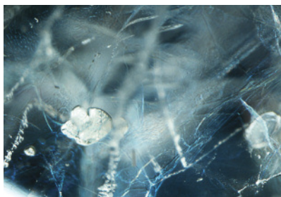
Figure 13. Flattened gas bubbles and a blue flash effect suggest that this stone contains significant amounts of lead glass, which was confirmed by EDXRF spectroscopy. Field of view 1.57 mm.
