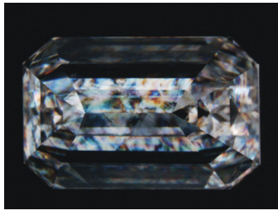
Figure 15. Viewed under crossed polarizers, this synthetic diamond shows mottled strain, but no tatami strain, consistent with its CVD growth origin.
