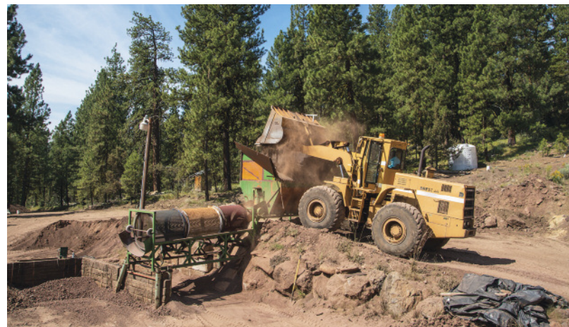
Figure 7. This loader transfers crushed basalt ore to a dry trommel, separating rock and feldspar crystals from the decomposed basalt, which is essentially dirt. Photo by Robert Weldon.
