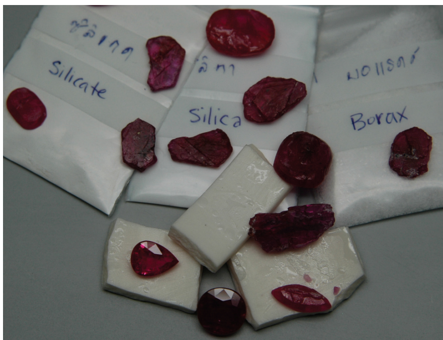
Figure 1: The three different powders used in the process, remnants of a ceramic crucible and some of the untreated and treated samples examined in this study. Photo: N. Sturman.
