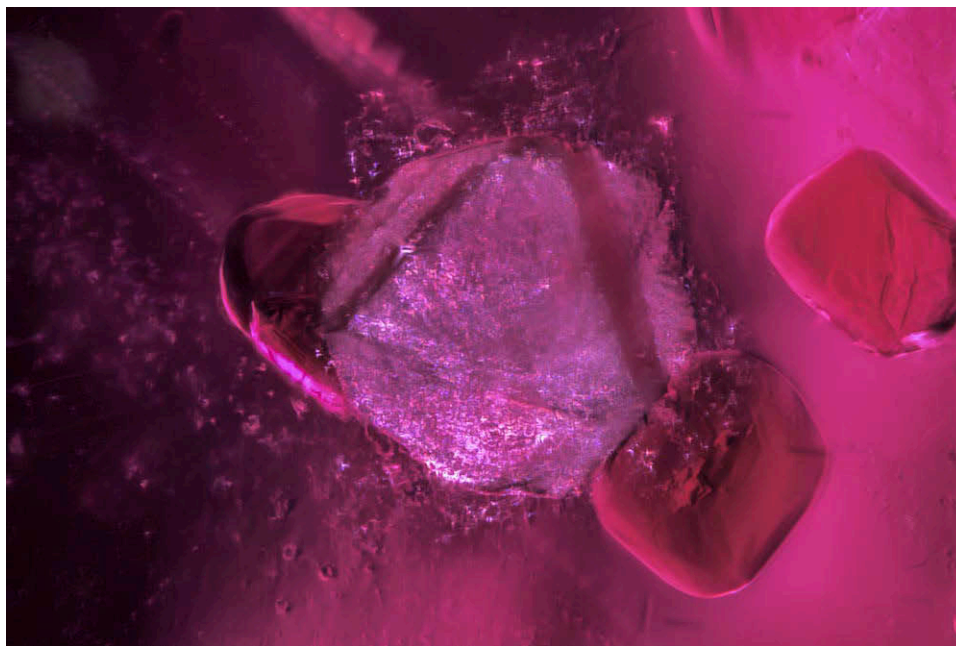
Figure 21. Orangy red staurolite crystals surround a negative crystal in a Mozambique ruby. Planes of thin films can be seen behind them. Photomicrograph by Nicole Ahline; field of view 1.42 mm.
