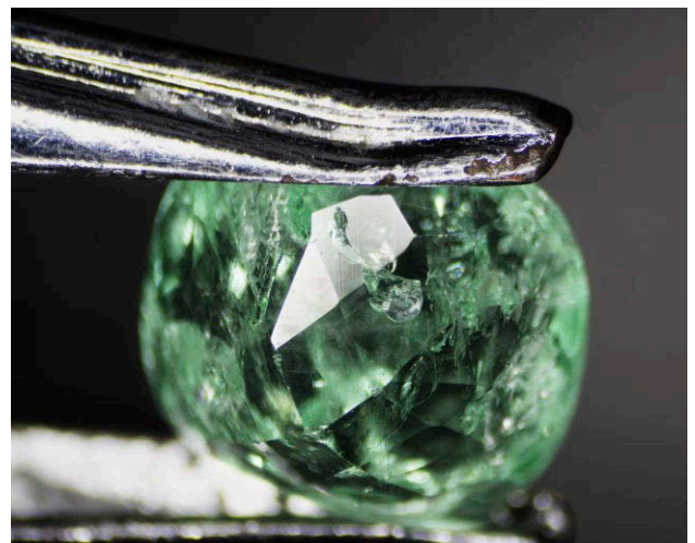
Figure 1. Fiber inside a cavity filled with liquid resin in a cushion-cut emerald measuring 8.2 \times 7.3 \times 3.1 mm. Photomicrograph by Holman Alvarado.
