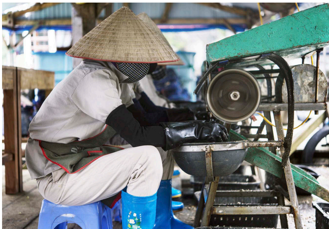
Figure 5. A POL staff member working on a series of wheel grinders to knock off surface growth from each shell. Photo by Nuttapol Kitdee.
