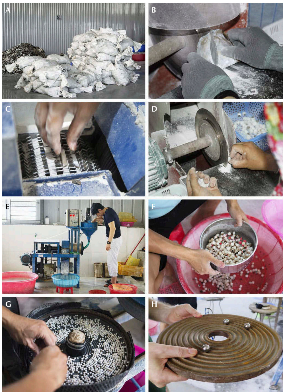
Figure 3. Photos from inside the factory showing the stages of nuclei production.
