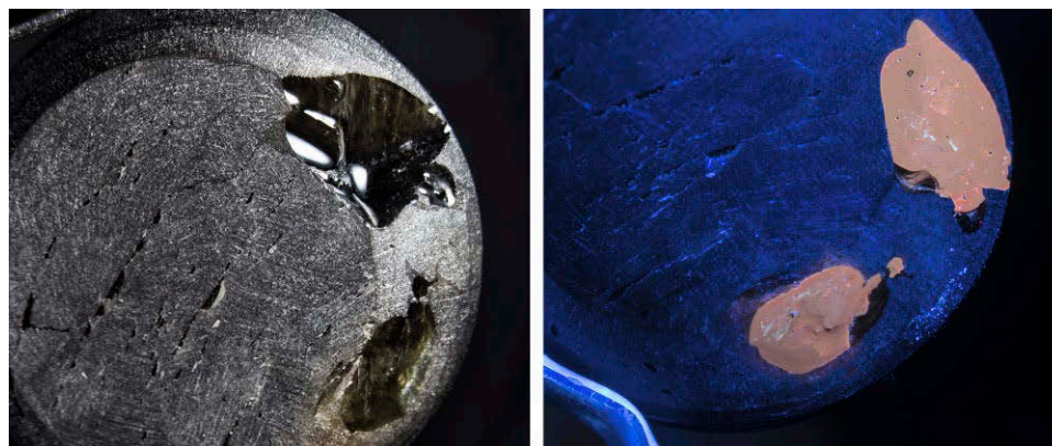
Figure 12. Left: Two large pits on the base of the star sapphire contain brown dopping varnish (the white areas are adhesive from tape). Field of view 30 mm. Right: Under long-wave ultraviolet light (365 nm), the dopping shellac fluoresced bright orange. Field of view 27 mm. Photomicrographs by Richard W. Hughes.
