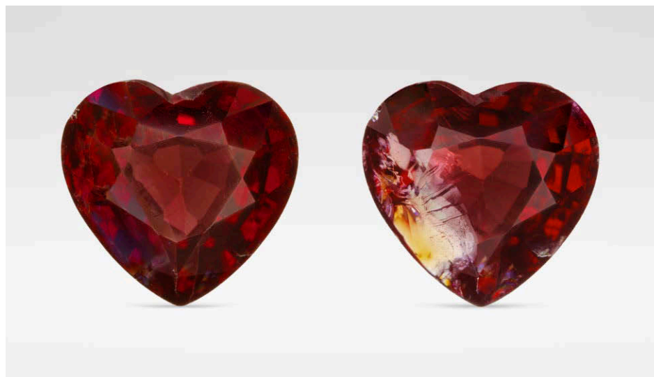
Figure 16. On the left is the 3 ct spinel as initially submitted. At right is the same stone after removal of the oil. The difference is striking. Following cleaning, a large reflective fissure is visible parallel to the girdle plane. This demonstrates the ability of an oil/resin to mask fissures even when there is no close match in refractive index between the filler and host. Photos by Chanon Yimkeativong/Lotus Gemology.
