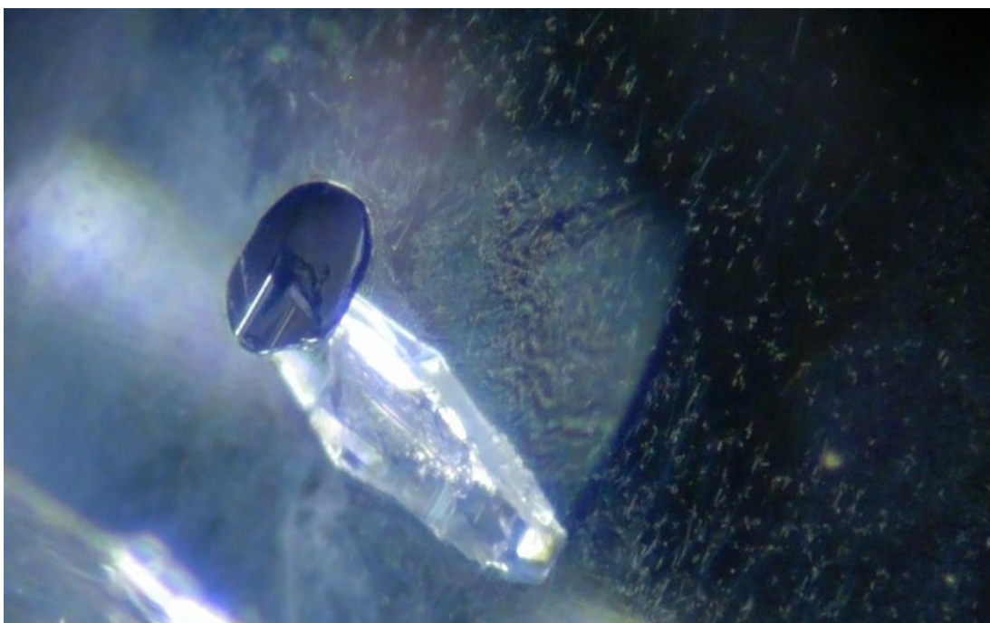
Figure 83: Negative crystal, graphite platelet, and particles and needles. Darkfield and fiber optic illumination, magnified 50x.
