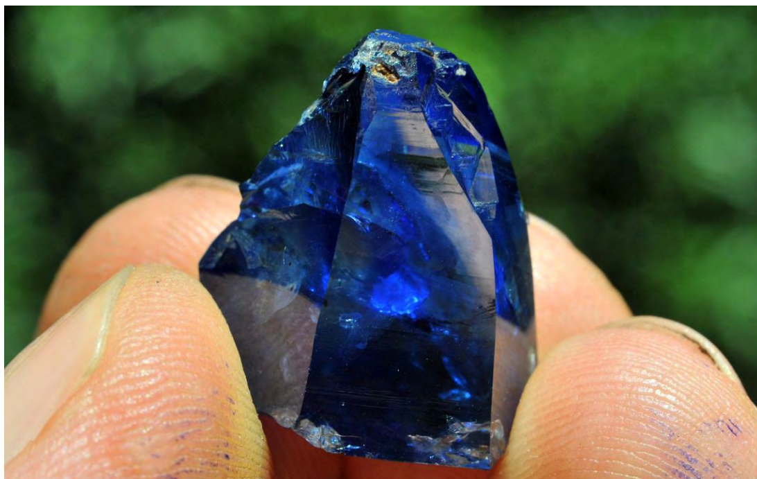
Figure 44. This sapphire crystal from Kataragama weighs approximately 46 carats. Note the strong color banding and colorless areas following the faces of the hexagonal bipyramid. Also note the numerous unhealed fissures. Photo: V. Pardieu / GIA Laboratory Bangkok.
