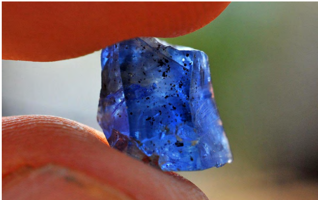
Figure 43. This 15 carat sapphire displays numerous opaque black inclusions. Photo: V. Pardieu / GIA Laboratory Bangkok.
