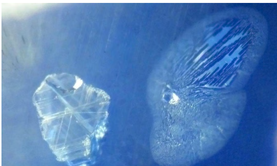
Figure 58: Negative crystals and healed fissure within GIA reference sample 100305162360. Darkfield illumination, magnified 50x.
