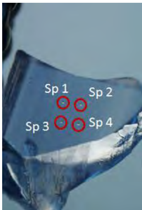
Figure 72: Four spots where LA-ICP-MS chemical data were obtained on the front of the wafer sample 100305161828. See Table 6.
