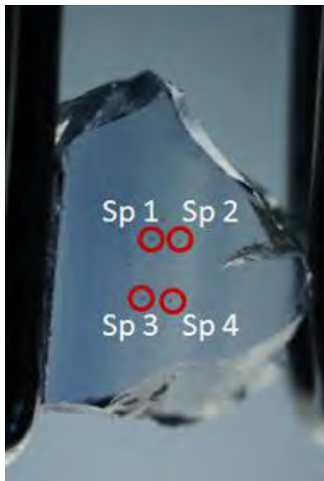
Figure 68: Four spots where LA-ICP-MS chemical data were obtained on the front of the wafer sample 100305161771. See Table 5.
