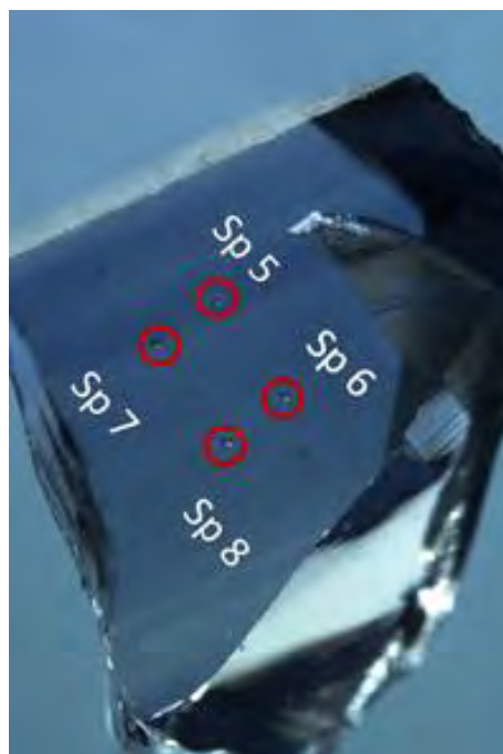
Figure 73: Four spots where LA-ICP-MS chemical data were obtained on the back of the wafer sample 100305161828. See Table 6.
