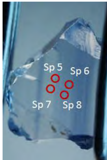
Figure 69: Four spots where LA-ICP-MS chemical data were obtained on the back of the wafer sample 100305161771. See Table 5.
