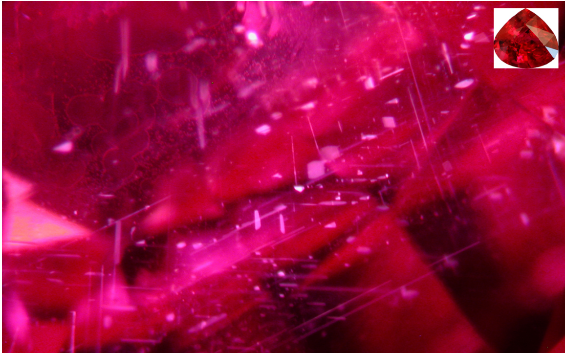
Figure 9, 2009: Silk in 1.054cts Niassa unheated ruby associated with unhealed fissures partially filled with dry foreign substance, probably of natural origin (Dark field illumination, 40x) Photo: V. Pardieu
