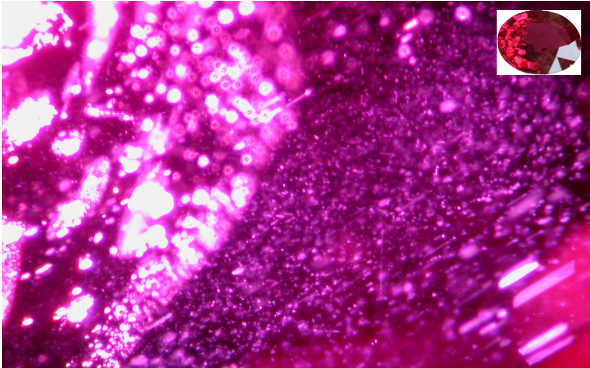
Figure 13: The same stone in the same position but this time using fiber optics illumination (30x): a galaxy of particles and needles, orientated perpendicular to the c axis, is now clearly visible. Photo: V. Pardieu
