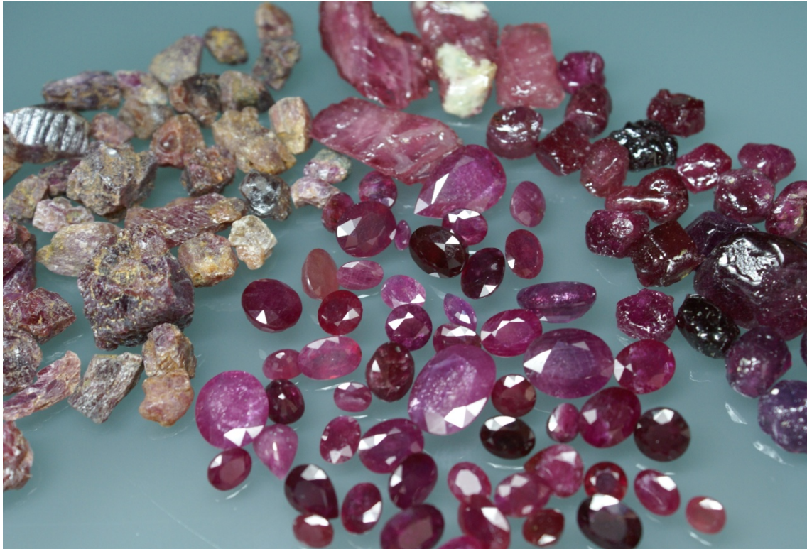
Figure 1: Some of the specimens used for this report. The rough specimens on the left represent the starting material, the specimens top and right represent the treated rough, and the specimens at center are cut from the treated rough.
