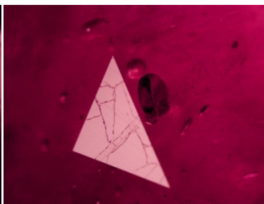
Figure 59:RGC010 showing wide and narrow tracts of glass crossing a facet in NTSR
