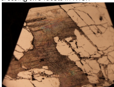
Figure 61:RGC014 showing wide tracts of glass crossing a facet in NTSR, The proportion of ruby to glass is in the region of 50/50
