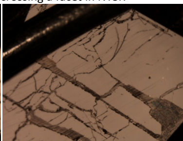
Figure 62: RGC014 showing wide tracts of glass crossing a facet in NTSR.
