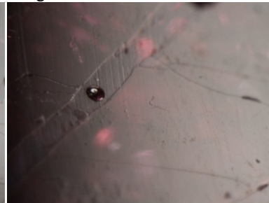
Figure 54 RGC002 showing a wide tract of glass crossing the table facet in NTSR, highlighted area on the same facet seen in Figure 52
