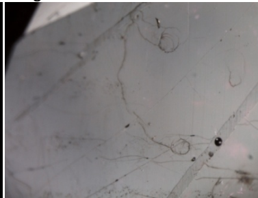
Figure 53: RGC002 showing a wide tract of glass crossing the table facet in NTSR, highlighted area on the same facet seen in Figure 52.
