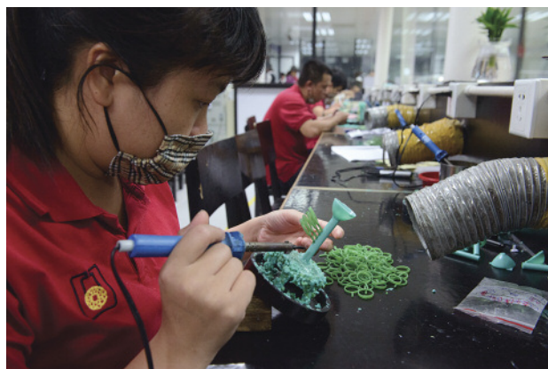
Figure 5. Hong Kong-based businesses have helped turn the Guangdong province into a major global manufacturing center. This jewelry factory uses modern manufacturing techniques such as wax models and casting. Photo by Eric Welch; courtesy of Chow Tai Fook.
