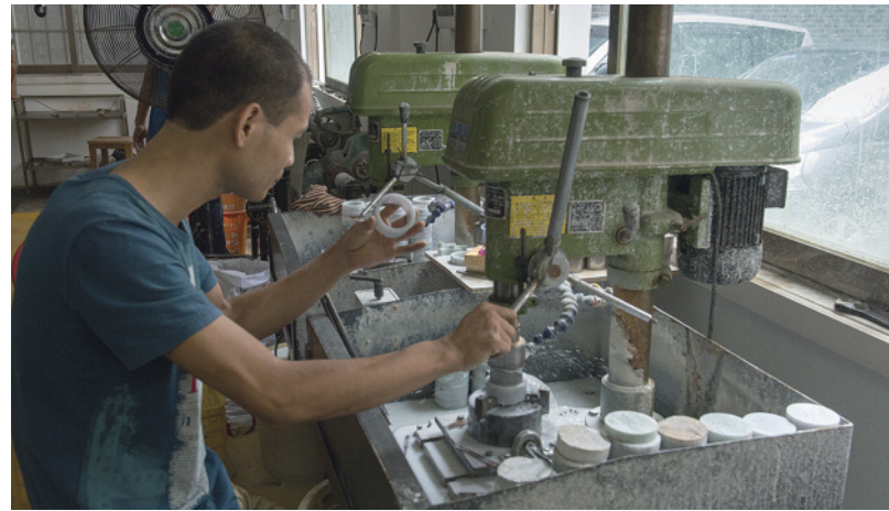
Figure 34. The Pingzhou area of Guangzhou is known for manufacturing jadeite bangle bracelets. This man is drilling the shape from a precut circular piece of jadeite. Photo by Eric Welch.
