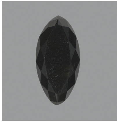
Figure 12. This 0.9 ct marquise proved to be a synthetic nanopolycrystalline diamond (NPD), the first one detected by a gemological laboratory.
