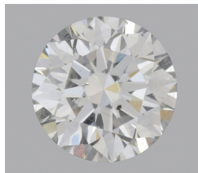
Figure 6. This G-color, 0.32 ct CVD-grown synthetic showed DiamondView features typically associated with a natural origin.
