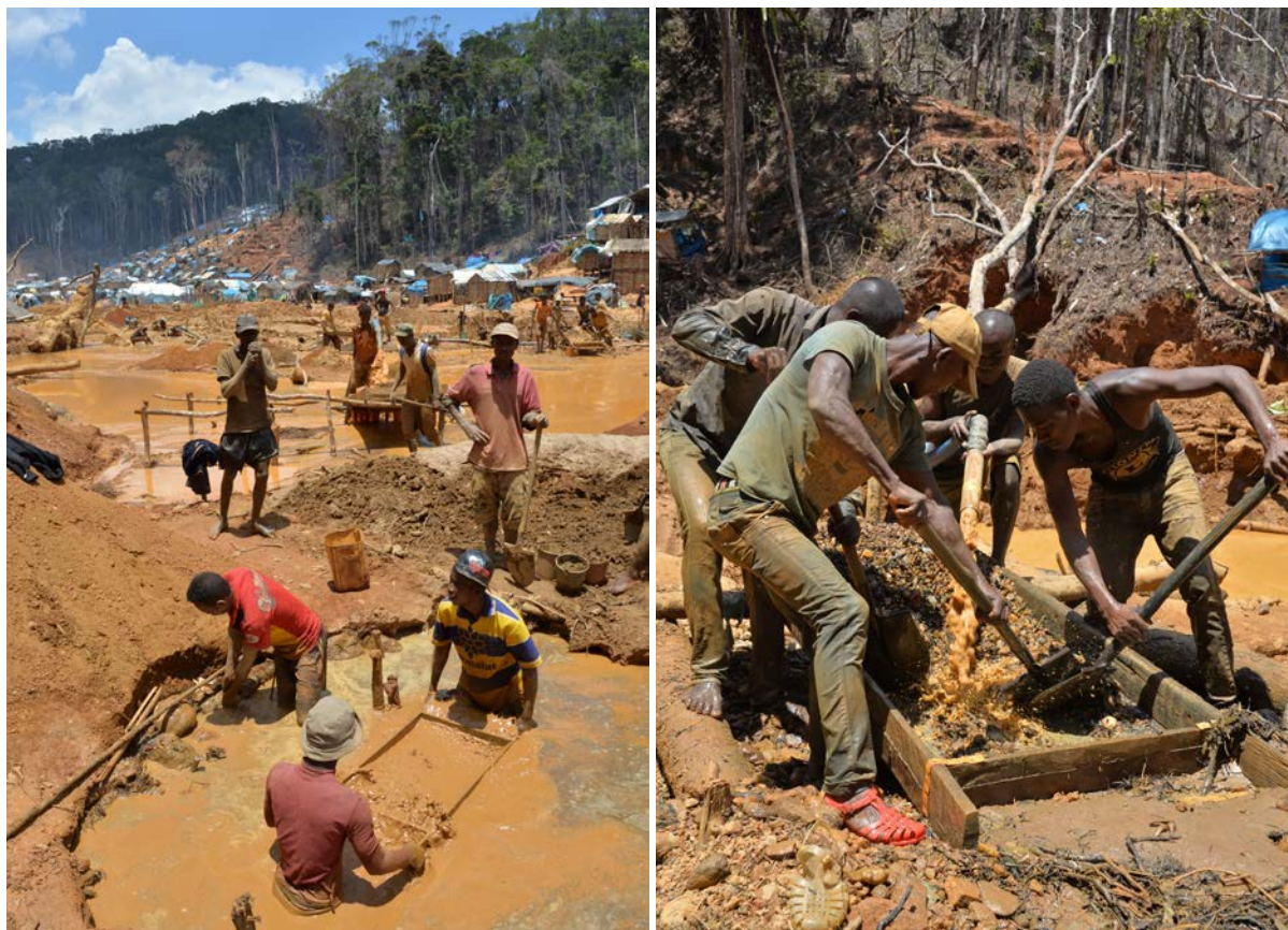
Figure 9: Malagasy miners working at Tananarivo Carrières (left) using the traditional hand sieves commonly found in Madagascar and at Milliard 1 (right) using the new method recently introduced here where teams of miners are working with a water pump, a hose and a large sieve. Photos © Vincent Pardieu, 2017
