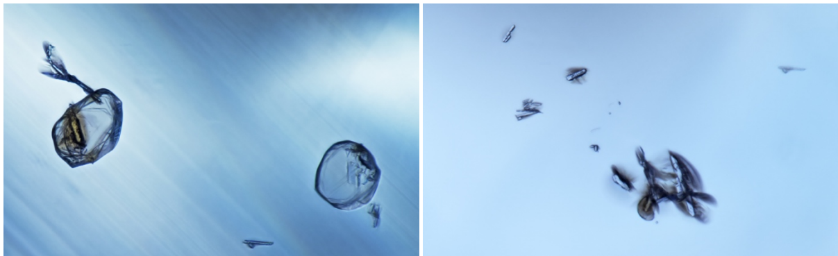
Figure 59: Left and right two different views on inclusions found in reference sample 100322689846 using bright field illumination. Left: Two tabular transparent crystals identified as mica with Raman and right: Few transparent crystals associated with unhealed tension fissures identified as zircon with Raman (using the RUFF database as reference). Field of view 1.20mm (left), 1.44mm (right), photos: Victoria Raynaud © GIA.
