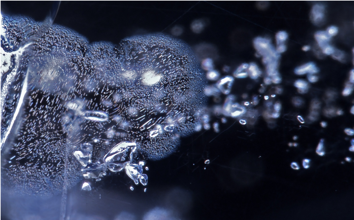
Figure 58: View of GIA reference sample xx841 using dark field, we can discover some healed fissures associated with a group of rounded transparent feldspar crystals. Field of view 1.12mm, photos: Victoria Raynaud © GIA.
