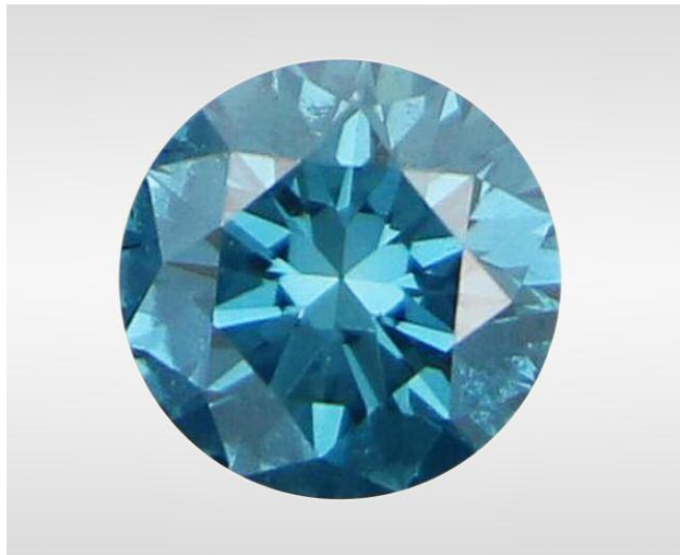
Figure 54. This 0.36 ct Fancy Deep green-blue diamond is a multi-step treated diamond. Photo by Wenqing Huang.
