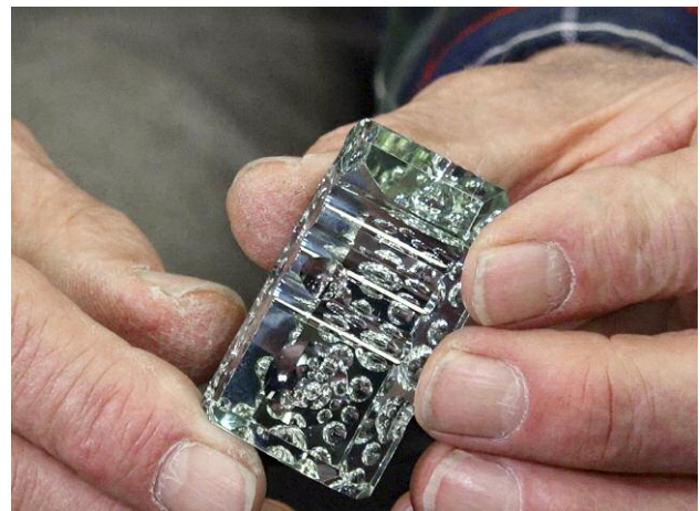
Figure 31. Each hole Dyber drills into a gem, as in this Brazilian green beryl, can take up to four hours to complete. Photo by Albert Salvato.
