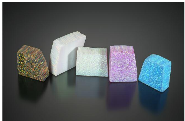
Figure 11. This new plastic opal imitation (left) shows a very pleasing play-of-color that does not have the classic “snakeskin” columnar structure one would expect to see in traditional polymer-impregnated synthetic opal produced by Kyocera (right). The largest sample of plastic imitation opal in the left photo weighs 227 grams, and the largest sample of synthetic opal in the right photo weighs 65 grams. The rectangular black block in the photo on the left is 9.7 cm in length.
