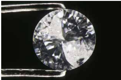
Figure 1. Large fractures in this diamond are exposed in high relief before treatment (left). After the fractures are filled, the same stone has a much improved apparent clarity (right).
