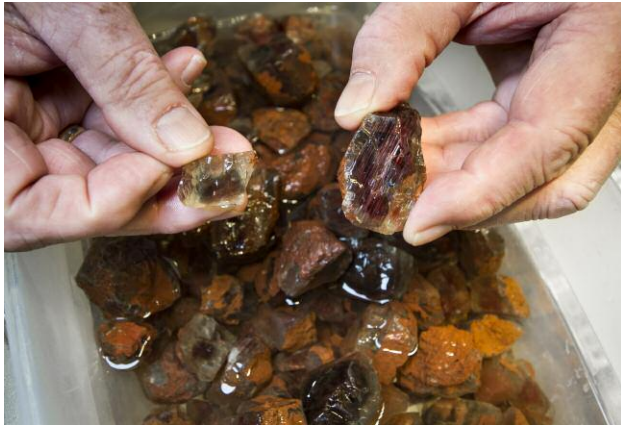
Figure 19. A new test pit on Desert Sun's Ponderosa claim has produced much larger rough, with a high proportion of large dichroic stones. The largest recovered so far was approximately 1,800 ct. Photo by Kevin Schumacher.
