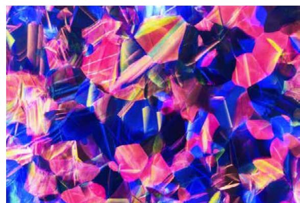
Figure 14. Randomly oriented patches of play-of-color are uniformly distributed throughout this new plastic opal imitation. The imitation looks the same from all different angles. Field of view 13 mm.
