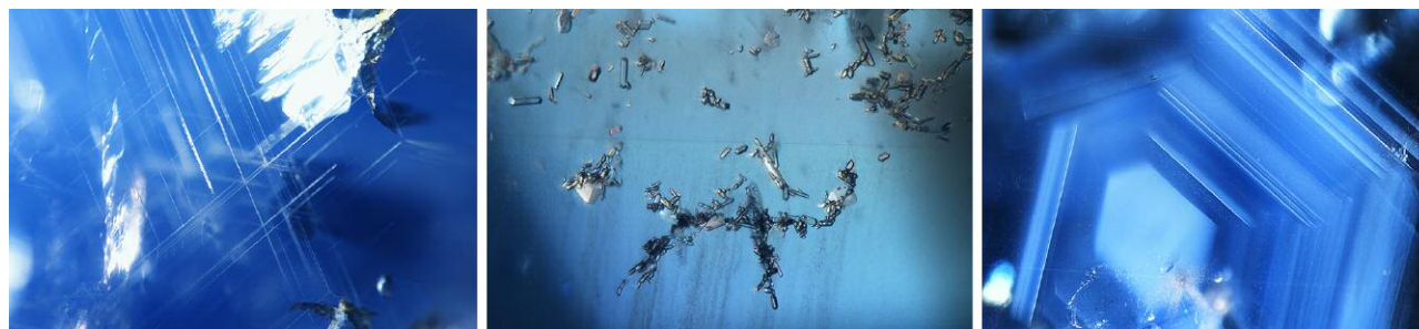
Figure 11. Left: Lamellar twinning with intersecting growth tubules under fiber-optic illumination; field of view 3.6 mm. Center: Cluster of zircon; field of view 1.8 mm. Right: Angular band of minute particles under fiber-optic illumination; field of view 3.6 mm. Photomicrographs by Charuwan Khawpong.
