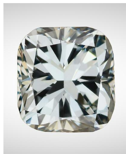
Figure 17. Face-up image of the natural diamond with CVD synthetic diamond overgrowth. The blue color is due to the boron-doped CVD layer.
