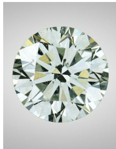
Figure 22. This 0.50 ct HPHT synthetic diamond, color equivalent to Faint Green, owed its color to nickel impurities.
