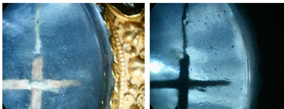
Figure 5. Reflected light (left) and transmitted light (right) reveal an abundance of bubbles in the glass cabochon. In both photos, the wooden cross and the silk thread are clearly visible. Photos by G. Panczer.
