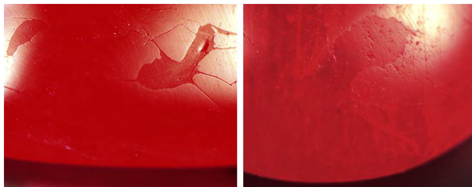
Figure 31. Notable differences in the reflectance of the glass filling and corundum host were seen in the DiamondView's visible light mode.
