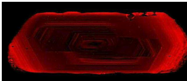
Figure 18. Raman photoluminescence mapping produced this image, which shows the relative distribution of chromium in a Yogo sapphire viewed perpendicular to the c -axis. Chromium is concentrated in the outer portion of the crystal and is not particularly homogeneous throughout. Field of view approximately 4 mm.
