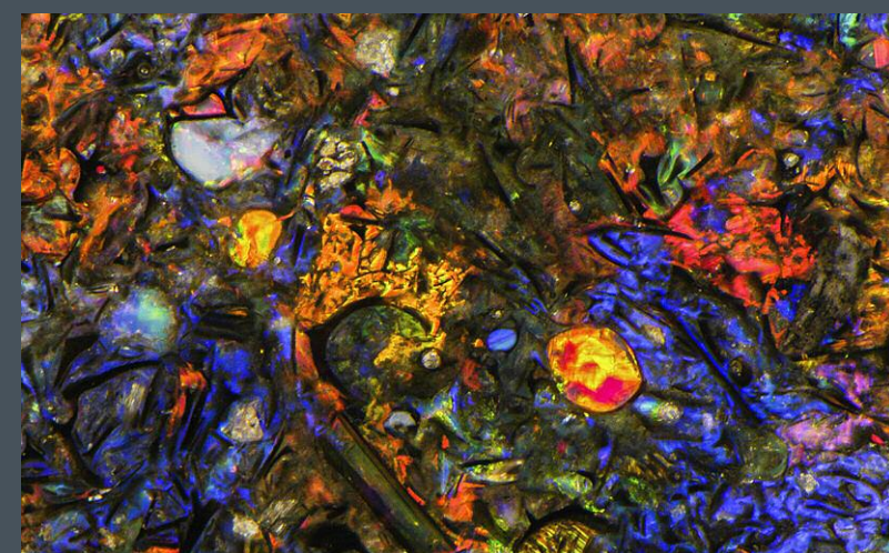
This Honduran opal formed in a natural porous volcanic rock that has been infilled with precious opal by a secondary process. Although the black bodycolor is natural, this stone is polymer impregnated to fill in surface voids and pits. Field of view 2.79 mm.
