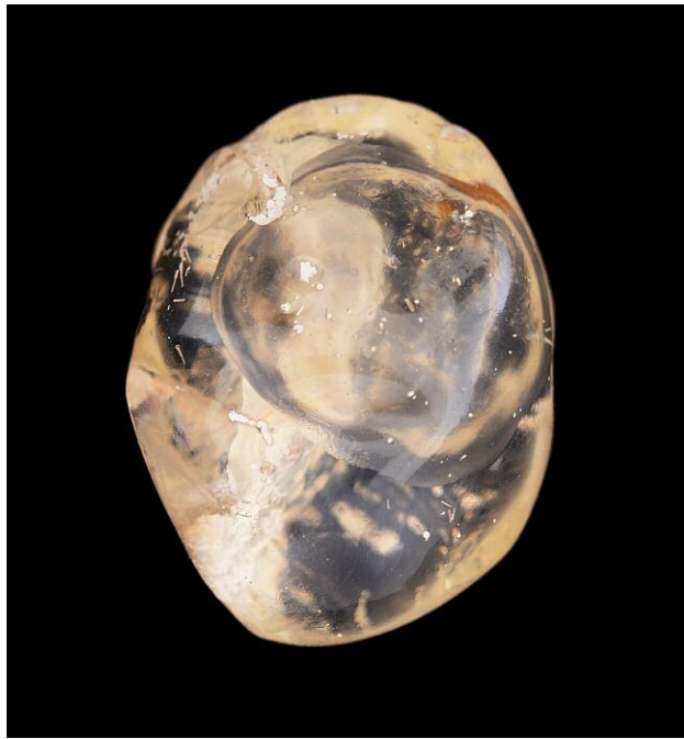
Figure 5. This 19.94 ct polished freeform opal contained a large, eye-visible three-phase fluid inclusion. Photo by Jian Xin (Jae) Liao; courtesy of Javier Lopez Ávila.
