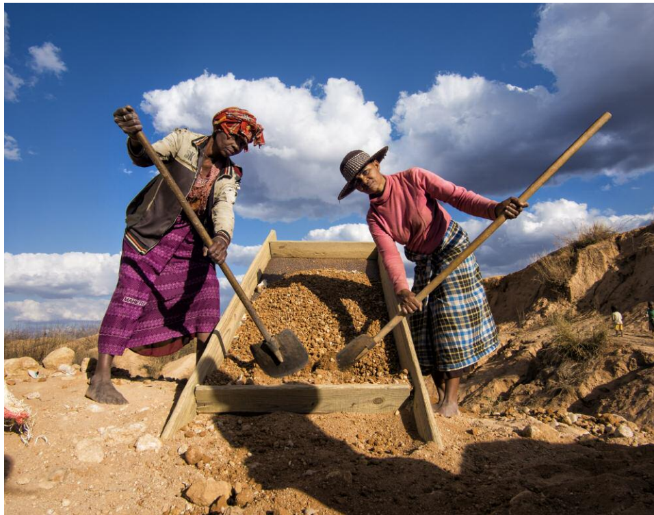
Figure 3. Miners move gem-bearing gravel near Ilakaka. Most of the sapphire production in Madagascar is by small-scale miners working with artisanal tools. Photo by E. Billie Hughes.
