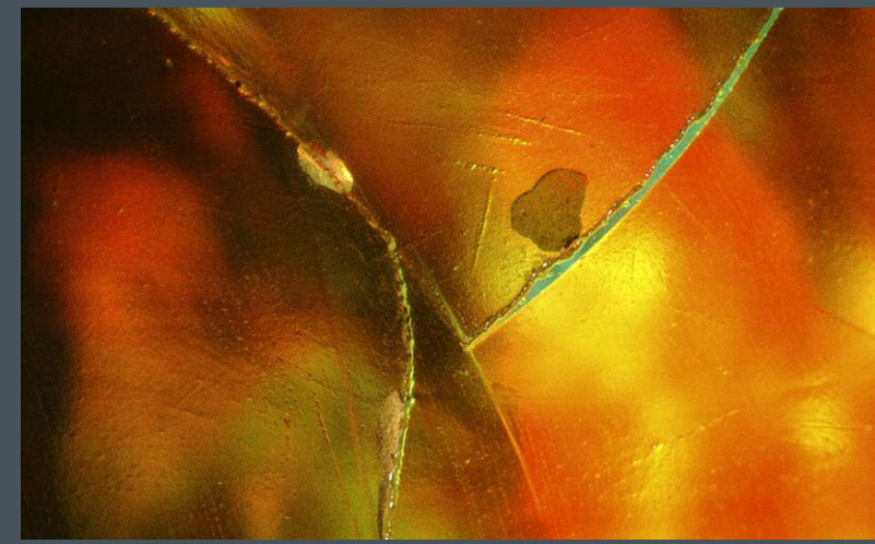
Some opals are prone to crazing or cracking, which can be hidden by filling the cracks with oil or resin. Trapped bubbles in the cracks of this opal reveal the treatment. Field of view 2.15 mm.
