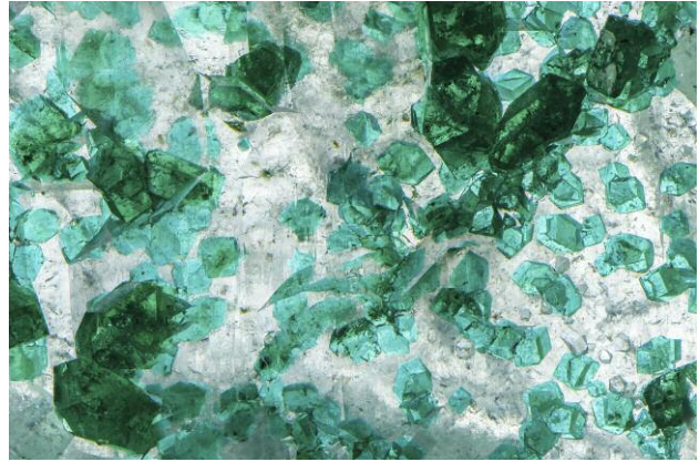
Figure 18. Trigonal blue-green crystals in and on the surface of this colorless quartz were identified by Raman analysis as diopside. Photomicrograph by Nathan Renfro; field of view 11.75 mm.
