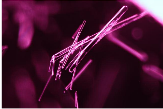
Figure 17. In some cases, amphibole occurs as elongated rod-like crystals. Photo by C. Khowpong; field of view 1.41 mm. Darkfield illumination.
