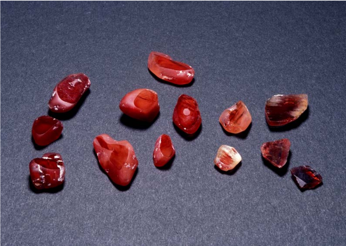
Figure 12. This pile of andesine rough (behind) was collected from the Bainang mine in Tibet. These untreated rough materials had a range of color and size (2.4-34.42ct), and they displayed rounded shapes and a water worn appearance. Parallel window were polished on samples examined for this study. Photo by M. Kobayashi.
