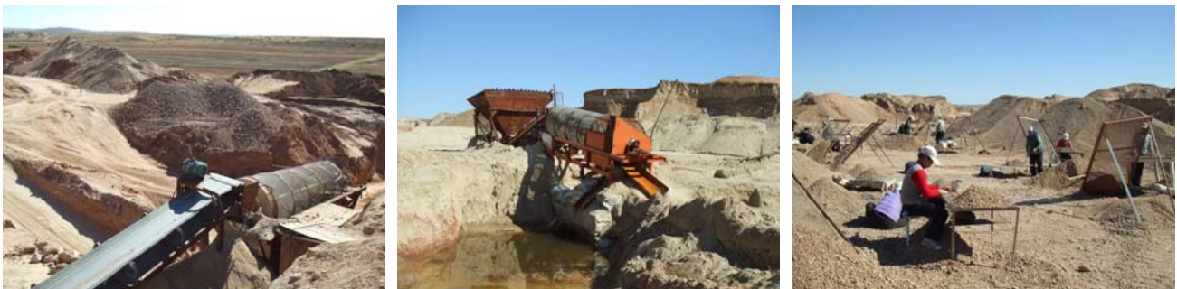
Figure 9. Future mining for yellow andesine by a Chinese company at Shuiquan (left) and Haibozi (center) in Guyang prefecture, Inner Mongolia. Andesine occurs in the secondary deposit of sand and gravel. Wet-screen selecting and hand picking of rough is performed onsite by miners (right). Photos by A. Abduriyim.
