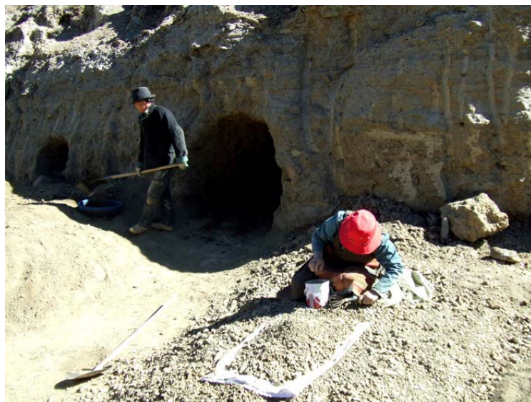
Figure 6. The andesine is excavated from a series of tunnels by local Tibetan miners using simple hand tools. Photo by A. Abduriyim.
