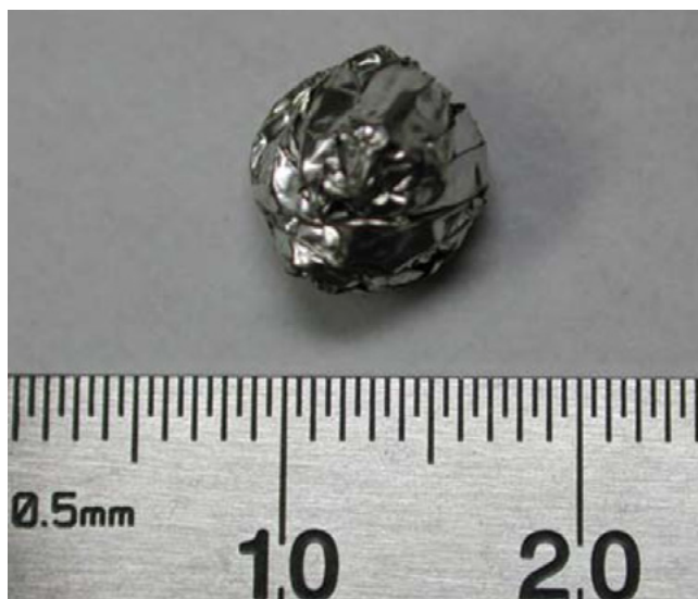
Figure 4. Sample wrapped in aluminum foil for argon extraction in the furnace. Photo by George R. Rossman.
