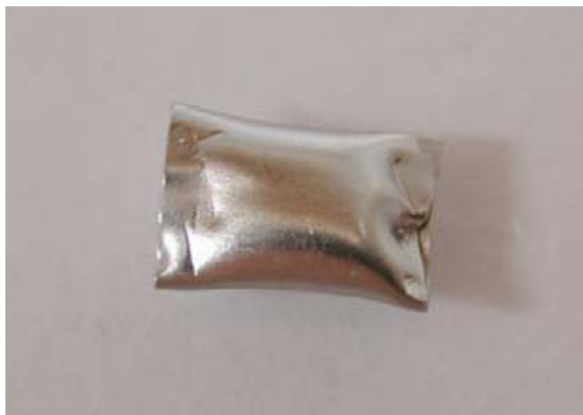
Figure 2. Platinum capsule containing about 20 mg of crushed andesine for argon isotope analysis. Photo by George R. Rossman.
