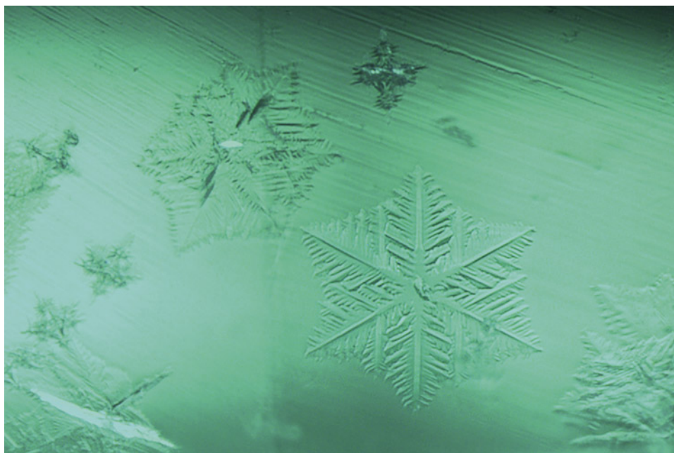
Figure 3. Brightfield illumination reveals a dendritic pattern in the star-shaped platelets, which bear a striking resemblance to snowflakes. Smaller three-dimensional crystal inclusions are also observed in the artificial glass. Photomicrograph by Kanako Otsuka; field of view 1.58 mm.
