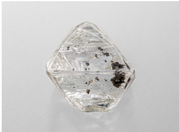
Figure 11. Weighing 2.34 ct and measuring 7.71 mm in the largest dimension, this partially etched diamond octahedron hosts a yellow-orange almandine-pyrope garnet crystal. Photo by Diego Sanchez.
