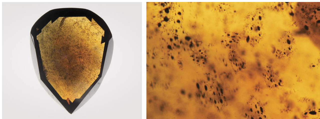
Figure 7. Left: A 1.03 ct Fancy Dark brown diamond containing carbon dioxide showing a high density of dark inclusion clusters. Right: The dark inclusions are larger (up to 50 \mu\text{m} ) than those observed in typical 480 nm band diamonds without detectable carbon dioxide (generally <10\text{ }\mu\text{m} ). Photos by Mei Yan Lai; field of view 1.26 mm (right).
