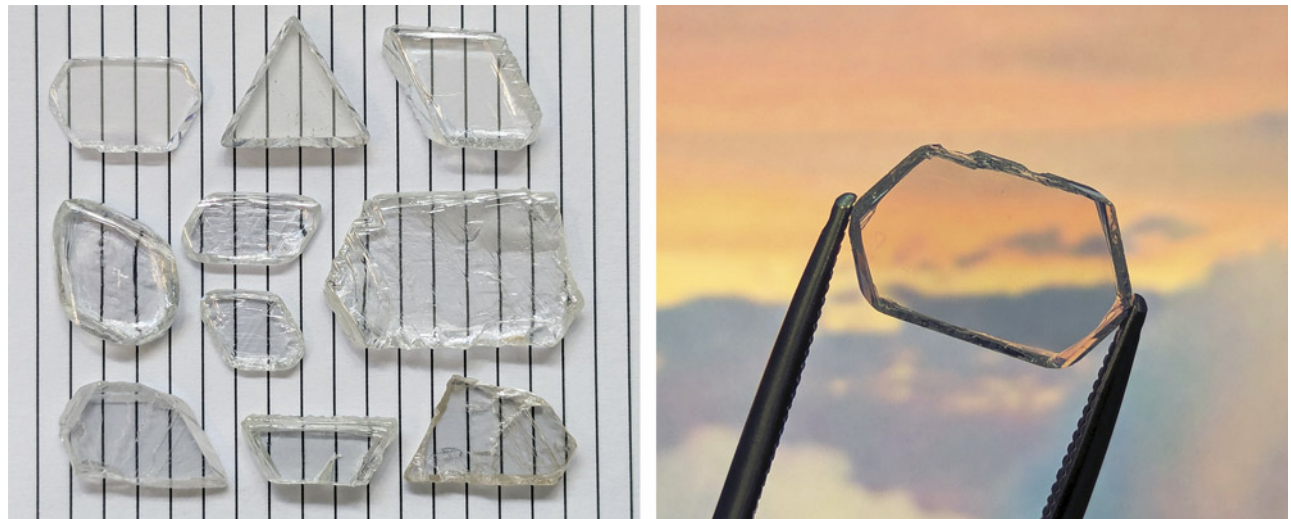
Figure 2. Left: Transparent plate-shaped rough diamonds ranging from 0.99 to 9.67 ct. Ruled lines have 2.8 mm spacing. Right: The top left specimen (2.22 ct) against the sky. Photos by Evan M. Smith.
