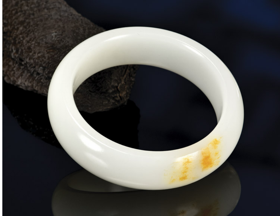
Figure 1. A high-quality Russian white nephrite bracelet, measuring approximately 58 × 13 × 7 mm, with the orange peel effect observable in its reflective areas. Photo by Zuojiang Chen.
