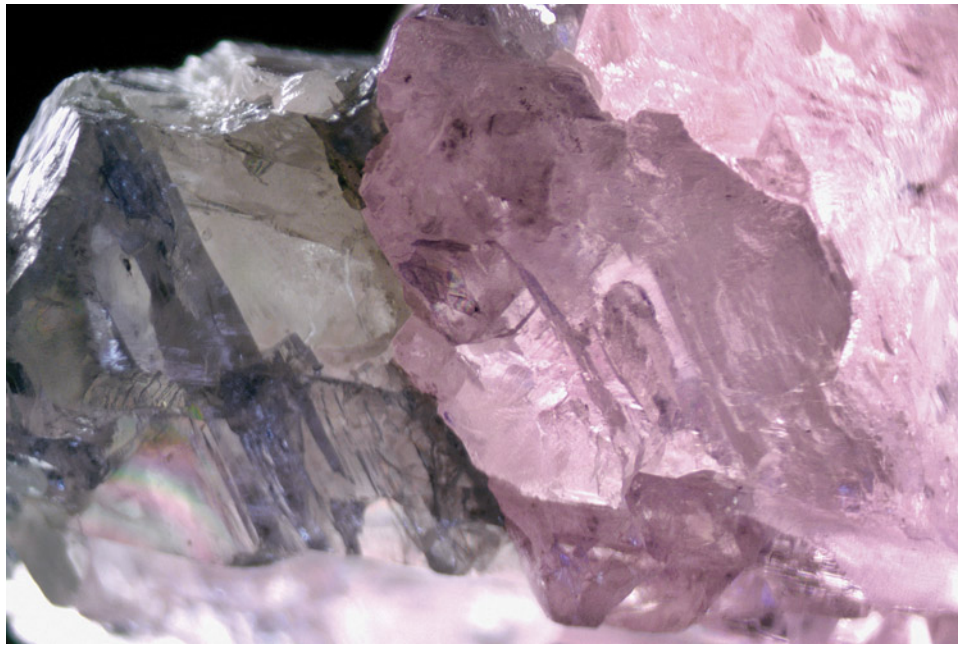
Figure 2. This boundary shows a sharp transition from pink to colorless zones. Photomicrograph by Wanling Tan; field of view 4 mm.
