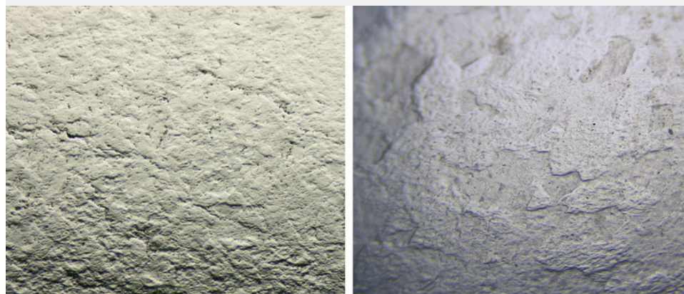
Figure A-1. The orange peel effect on the surface of jadeite from Guatemala (left) and nephrite from Russia (right) viewed under oblique illumination. Photomicrographs by Meiyu Shih; field of view 6 mm.
