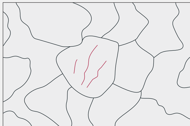
Figure A-3. A simple sketch showing the claw lineation pattern. The red lines represent claw lineation, and the outlined gray particles represent the granular microstructure (pseudomorphs) of nephrite.
