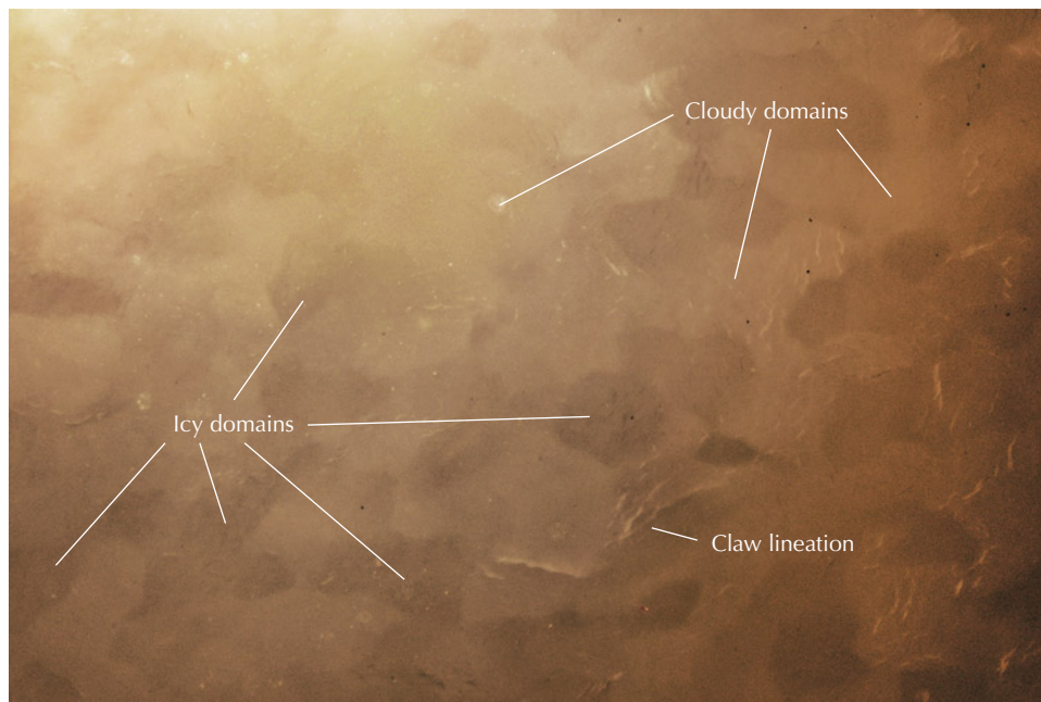
Figure 4. The polished surface of Russian white nephrite sample ELS27 showed icy domains (darker grains), cloudy domains (lighter grains), and claw lineation under oblique illumination with a sodium light source. Photomicrograph by Meiyu Shih; field of view 6.90 mm.
