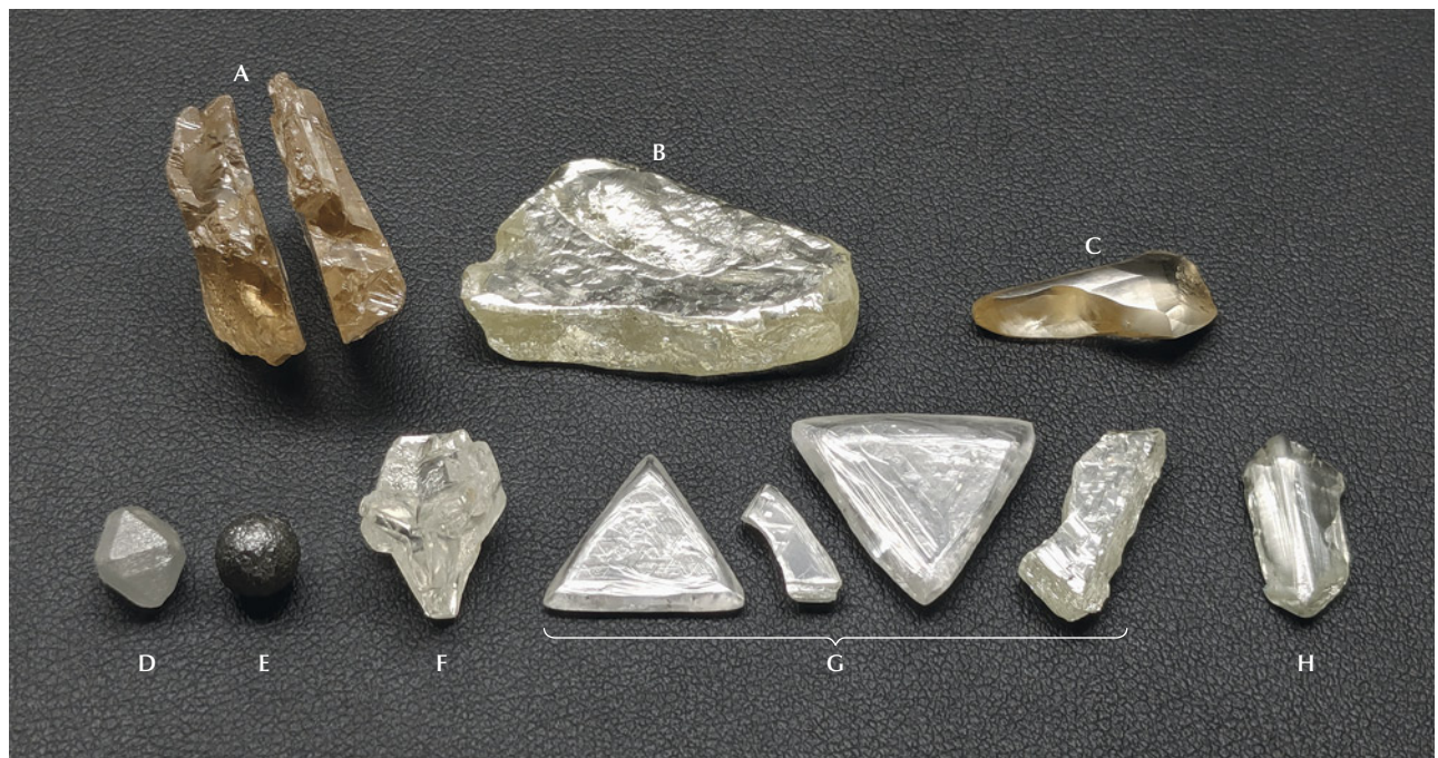
Figure 1. Examples of rough diamonds with shapes governed by various combinations of growth, breakage, and resorption: a diamond broken cleanly along a flat plane by cleavage (A); irregular broken fragments smoothed by resorption (B and C); cuboctahedron (D), ballas (E), and re-entrant cuboid (F) shapes produced during diamond growth; two macles resulting from twinned crystal growth, along with two fragments resulting from macle breakage (G); and an elongate fragment representing an edge broken from an octahedron crystal, with the former octahedron corners forming the ends (H). Specimens range from 1.08 to 28.08 ct, with the largest specimen measuring 27 mm in length. Photo by Evan M. Smith.
