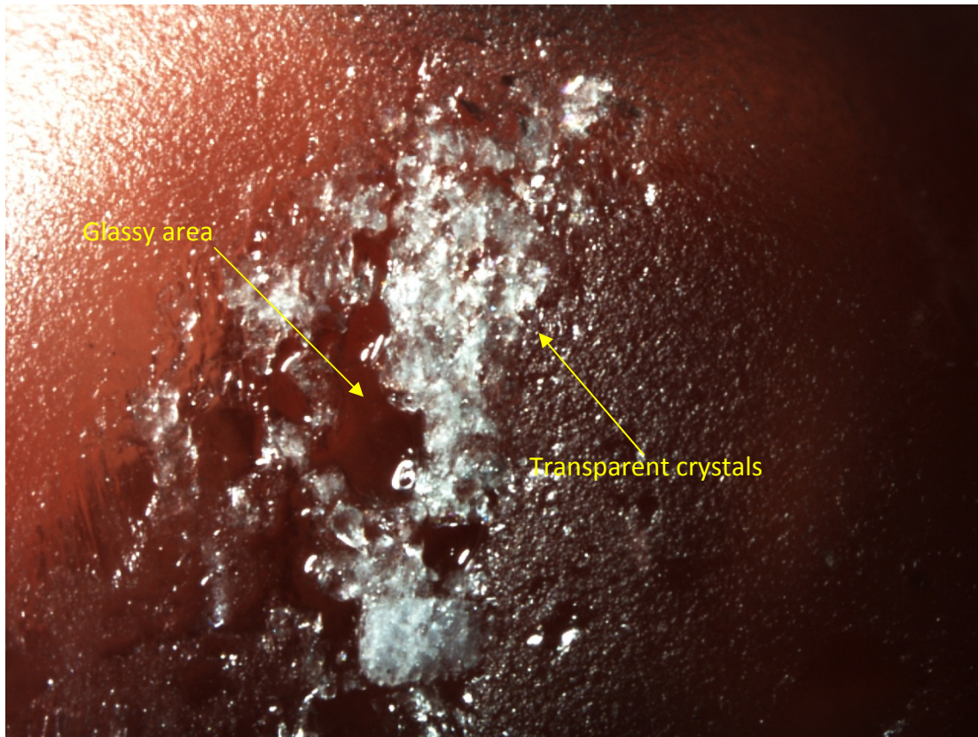
Figure 41 Surface of sample 17401909 from Tibet. The area appears melted with smooth glassy surface and clusters of transparent crystals. Photo by Garry Du Toit.
