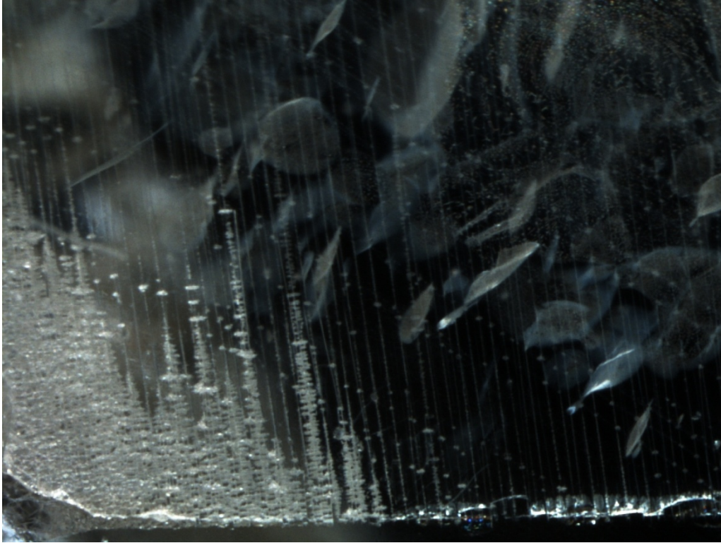
Figure 36: String of crystals with large discoid fractures which occurred after heating (668714602). See Figure 35, note the differences before heating.
