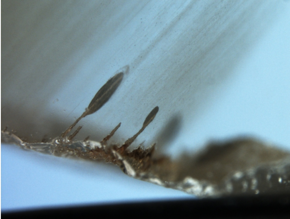
Figure 40:: A fracture appeared at the top after heating (668715202). See Figure 39, note the differences before heating.
