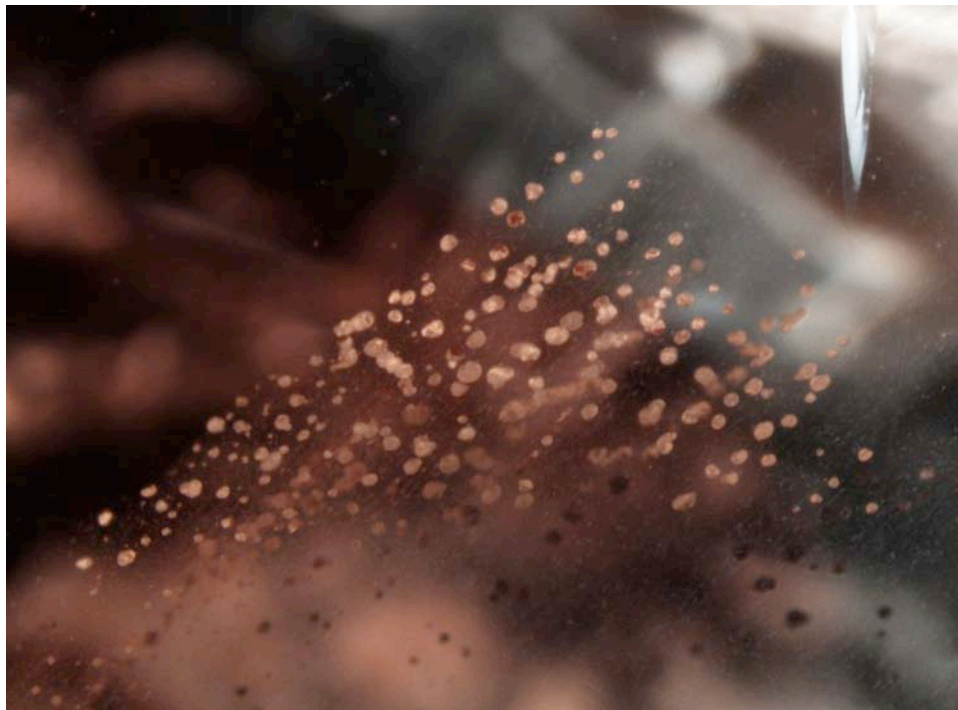
Figure 17. The eye-visible schiller in untreated Oregon feldspar is caused by relatively large copper platelets. Photomicrograph by Shane McClure.
