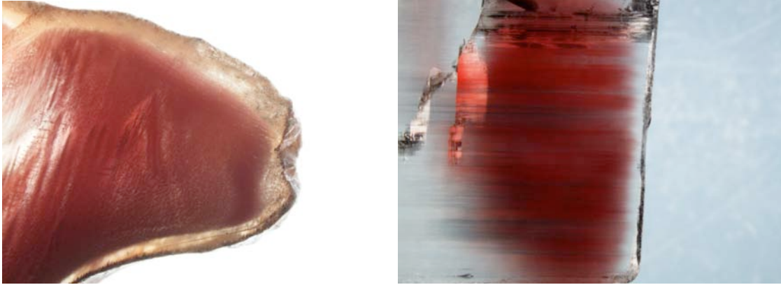
Figure 19. This colorless zone is present in treated (left) and untreated feldspar (right), regardless of the stone's origin or who treated it. Photomicrograph by Shane McClure.
