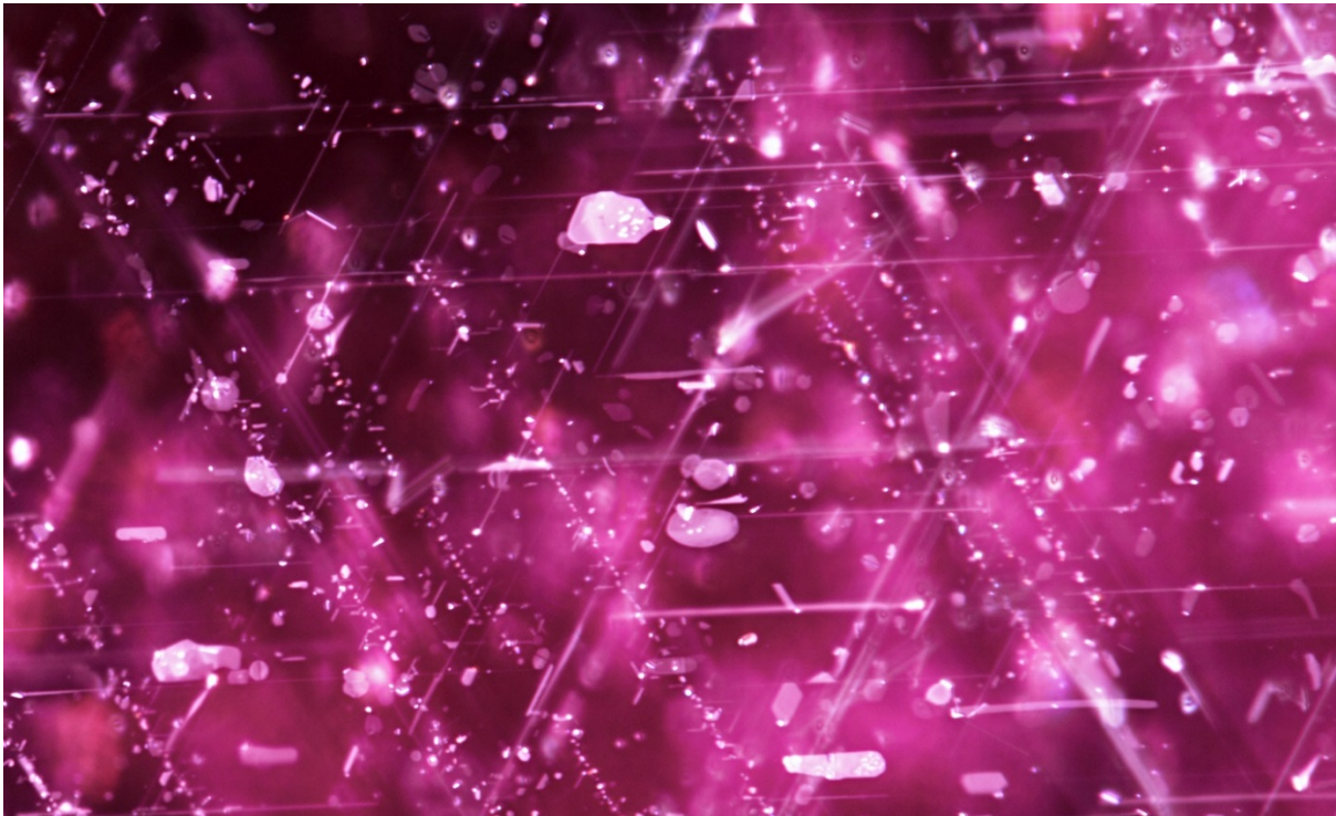
Mozambican ruby with spotted platelets that indicate heat treatment. Fiber-optic illumination. FOV 1.0 mm. Photo: C. Khowpong © GIA.
