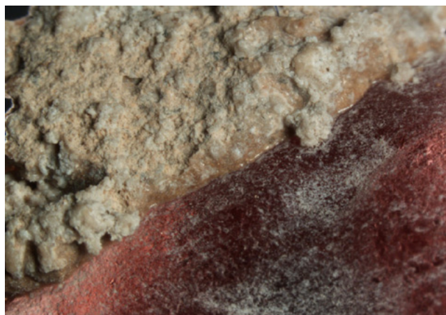
Figure 5 – In some cases the contact material formed a meniscus where the andesine and the matrix met. Photomicrograph by S. F. McClure. Field of view 2.1 mm.
