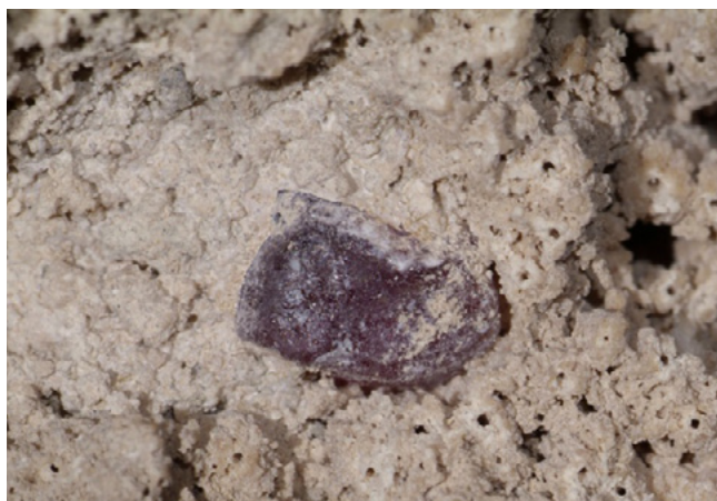
Figure 3 – The andesine embedded in the matrix had mostly rounded edges and frosted surfaces, indicating they had been worn by alluvial processes sometime before ending up in the matrix. Photo by S. F. McClure. Field of view approx. 25 mm.
