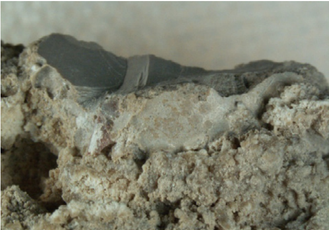
Figure 13 – The area around where the andesine had been attached showed a fine grained structure and had a somewhat glassy appearance that was entirely unlike the rest of the matrix. Photomicrograph by S. F. McClure. Field of view 4.5 mm.
