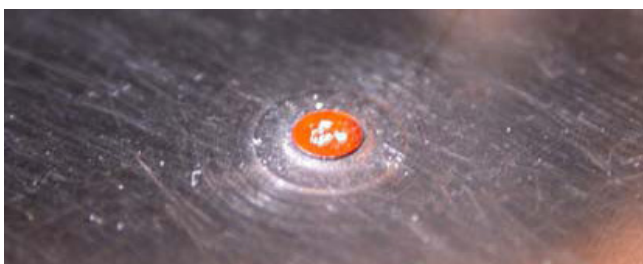
Figure 7. The contact material on the diamond plate of the ATR accessory. Photo by G. Rossman.
