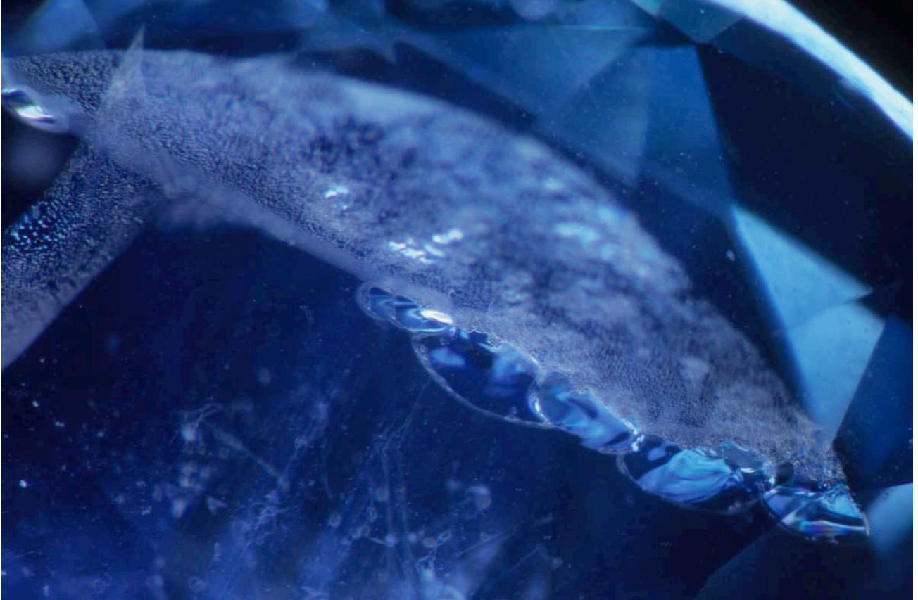
Figure 2. While it is not possible with current gemological microscopes to resolve the interior of any of the fluid inclusion islands in this “fingerprint,” the glassy fringe of microcracks along the edge provides evidence of high-temperature heat treatment. Such obvious visual information is not always present, however. Photomicrographs by John I. Koivula. Horizontal field of view is approximately 4 mm.
