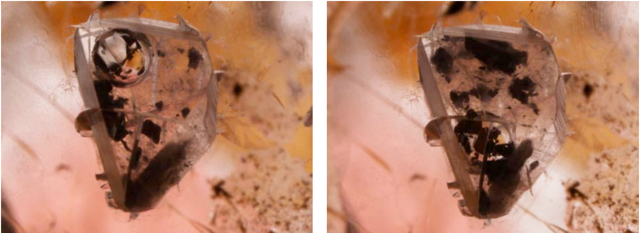
Figures 1A and 1B. Containing a mobile gaseous phase suspended in an aqueous fluid, with numerous graphite platelets also present as solid phases, this intact 1.86-mm-long primary fluid inclusion clearly shows that the host spinel could not have been heat treated. Photomicrographs by John I. Koivula.
