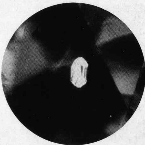
Figure 43 Individual zircon crystal with well- developed crystal faces, enclosed in a diamond. G.I.A. Dia- mondscope. 100x.
