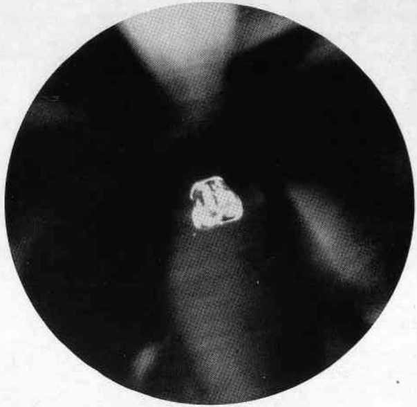
Figure 44 A diamond crystal of less symmetrical form than that in Figure 39, enclosed in a diamond. G.I.A. Diamondscope. 100x.
