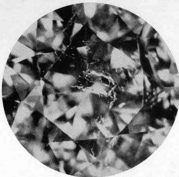
Figure 46 Irregular cracks and fractures below the table of a diamond. G.I.A. Diamond- scope. 22x.
