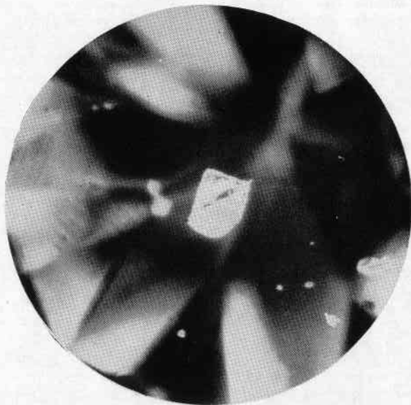
Figure 39 Included diamond crystal, the octahed- ral habit of which is distinctly seen, in a diamond. G.I.A. Diamondscope. 100x.
