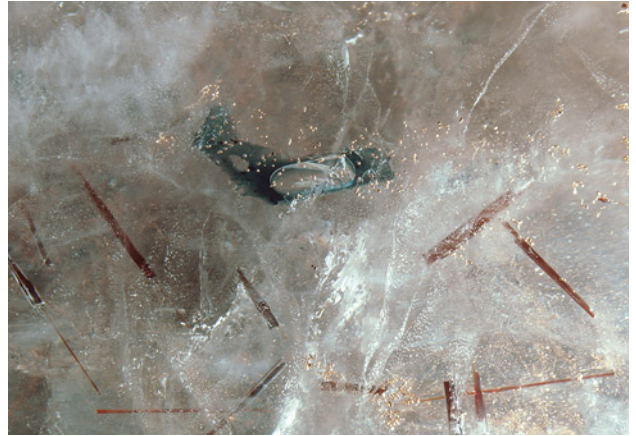
Figure 13. A suite of columbite rods, copper crystals, and a large air bubble seen within a film of blue flux liquid. Photomicrograph by Jamie Price; field of view 7.19 mm.
