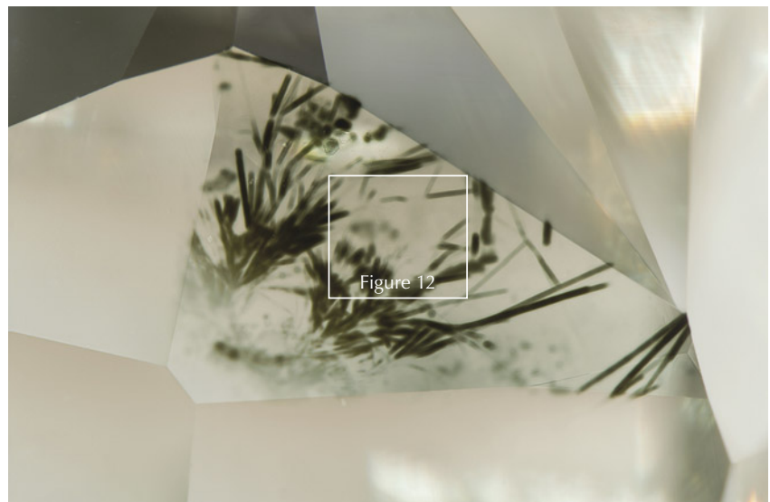
Figure 11. Blade-like green radiation stains. Also indicated is the boundary of the close-up view of the green stains in figure 12. Field of view 2.9 mm.
