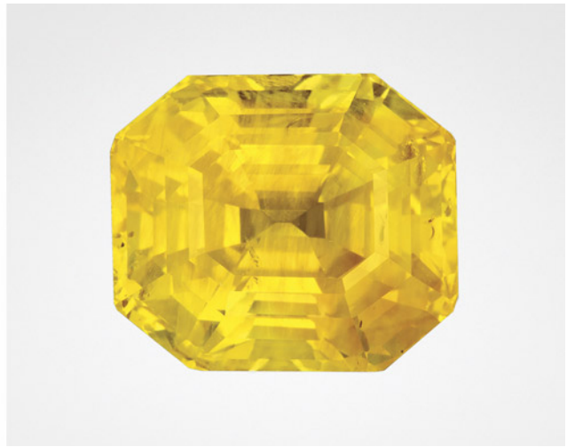
Figure 30. Left: Before a fade test, this approximately 10 ct sapphire displayed a strong orange hue. Right: After the fade test, the orange color became less pronounced and the stone appeared yellow. Photos by Ronnakorn Manorotkul.
