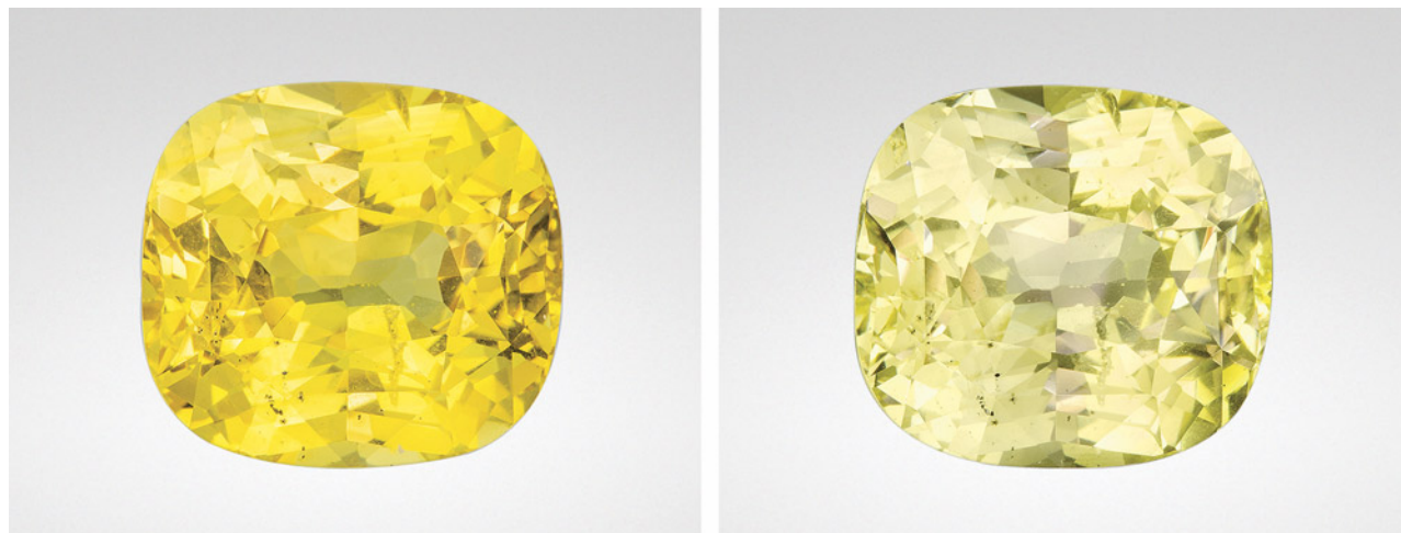
Figure 33. Before a fade test, the unheated sapphire of approximately 18 ct displayed a highly saturated yellow hue (left). After a fade test involving light and mild heat, the color faded to a pale yellow (right). Once the stone was exposed to sunlight for 30 minutes, the more intense yellow color displayed before the fade test came back. The sapphire was then subjected to a light-only fade test, and the more saturated yellow color remained stable. Photos by Ronnakorn Manorotkul.
