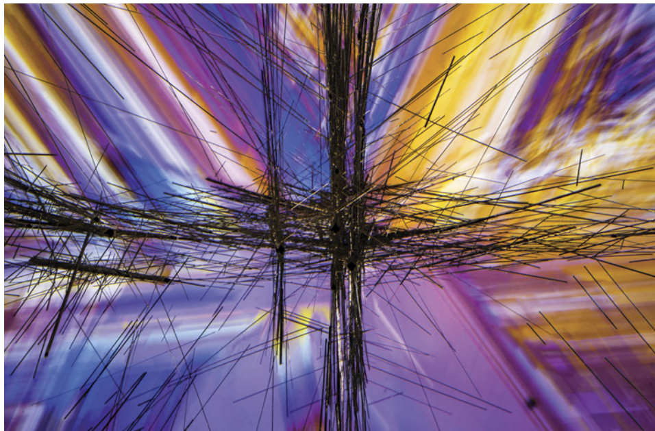
Figure 14. Rutile needle inclusions in a quartz host. Cross-polarized light shows off the Brazil-law twinning in the quartz, creating a spectacular display of light. Photomicrograph by Nathan Renfro; field of view 20.05 mm.
