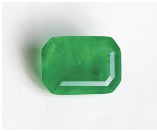
Figure 24. This 11.30 ct sample (18.9 × 14.0 × 8.8 mm) was found to be a triplet composed of colorless glass and quartz held together by green cement. Photo by Biqian Xing.
