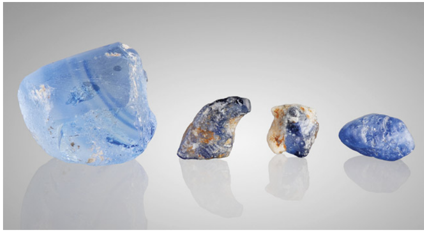
Figure 4. This set consists of a 48.63 ct piece of manmade glass (left), 9.17 and 6.21 ct laboratory-grown sapphires with resin imitation of matrix on the surface (center), and an 8.46 ct natural blue sapphire rough (right).
