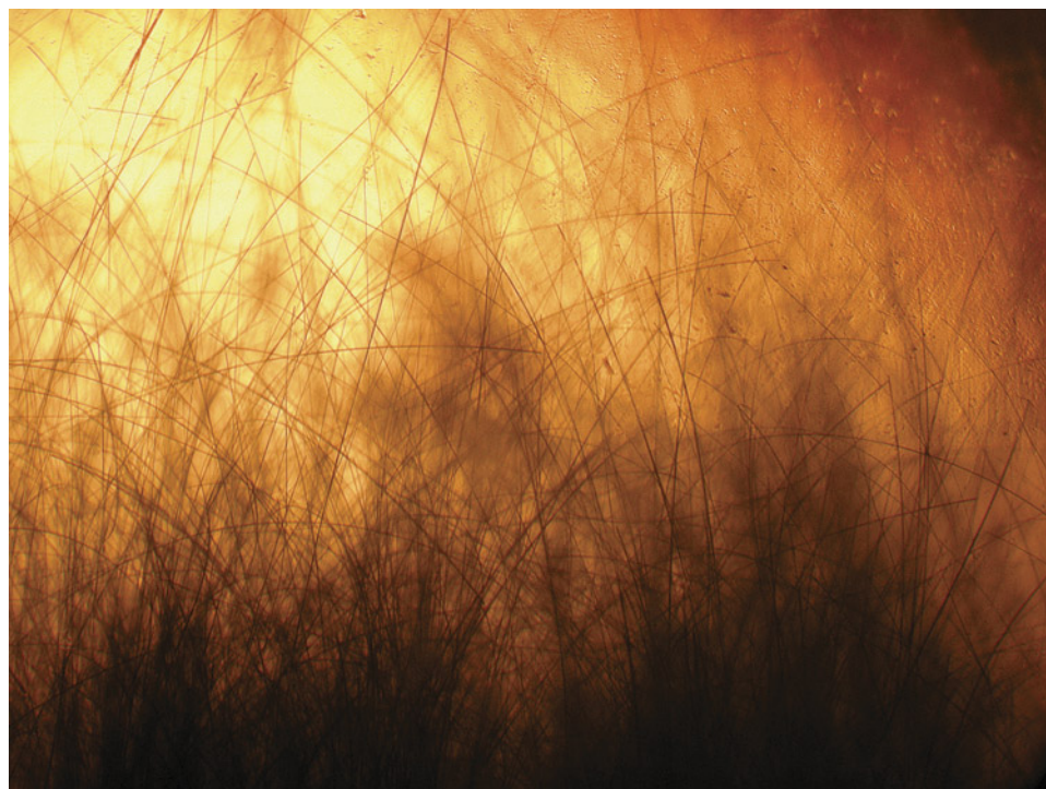
Figure 17. Fibrous inclusions in a quartz cabochon from Brazil showing three-rayed asterism. Photomicrograph by Karl Schmetzer; immersion, field of view 7.6 mm.
