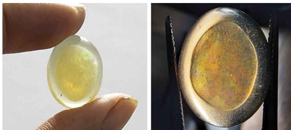
Figure 22. An 11.68 ct treated phantom opal in which the phantom structure appeared during experiments with various solutions. The sample is shown under daylight through the dome (left) and under halogen lighting through the bottom (right). Photos by Le Ngoc Nang.
