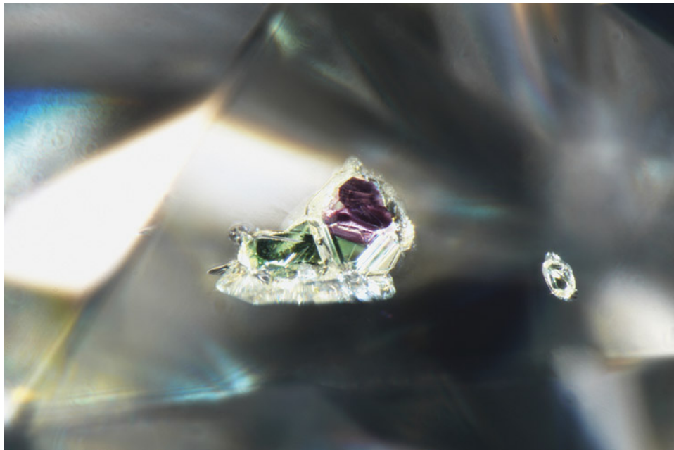
Figure 10. This “snail” inclusion was viewed through the upper half facet of a 4.00 ct near-colorless diamond. The purple-red “shell” was identified as pyrope garnet, while the green “body” was determined to be diopside. Photomicrograph by Christopher Vendrell; field of view 1.99 mm.
