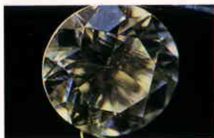
Growth striations in cubic zirconia. Magnification 10x.
