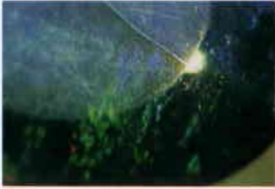
Plastic treated and dyed Brazilian opal showing hydrofluoric acid etch mark.
