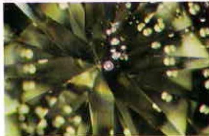
Large gas bubbles like these are rare in cubic zirconia. Magnification 45x.
