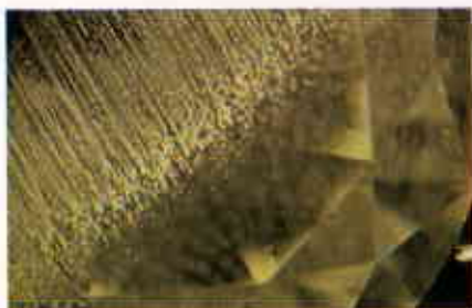
Stringers of negative crystal "gas bubbles." Magnification 25x.
