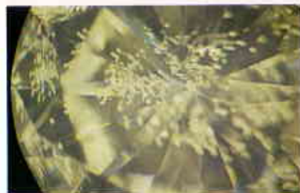
Elongated bubbles partially lined with flux. Magnification 15x.
