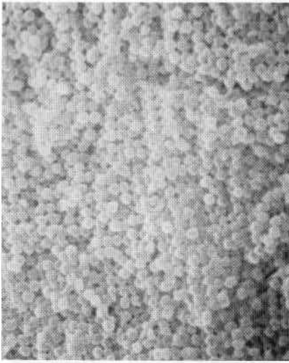
Scanning electron microscope view of etched surface natural Australian opal magnified 14,000x
